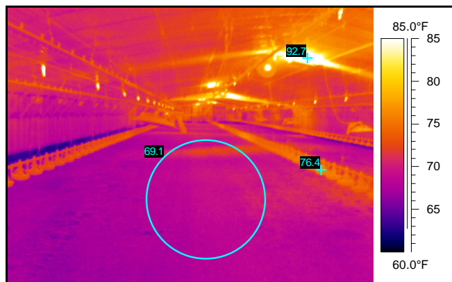
Figure 3. Thermal image of a house using attic inlets between flocks (springtime).
